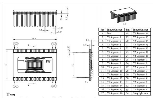
Outputs Y1, Y2 are interchangeable. The anodes Y1, Y2 must be at negative potential compared to the cathode (bias pin). The stray-light area should be connected to the same potential as the anodes.
